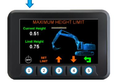
Button 1 Turns the limit ON or OFF. If turned on here the system uses the last saved Limit
